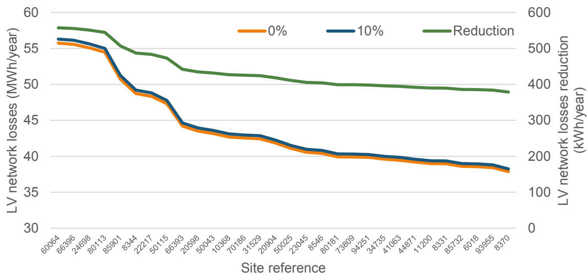
Figure 3.16. Impact of reducing total harmonic current distortion on losses at LV networks.
