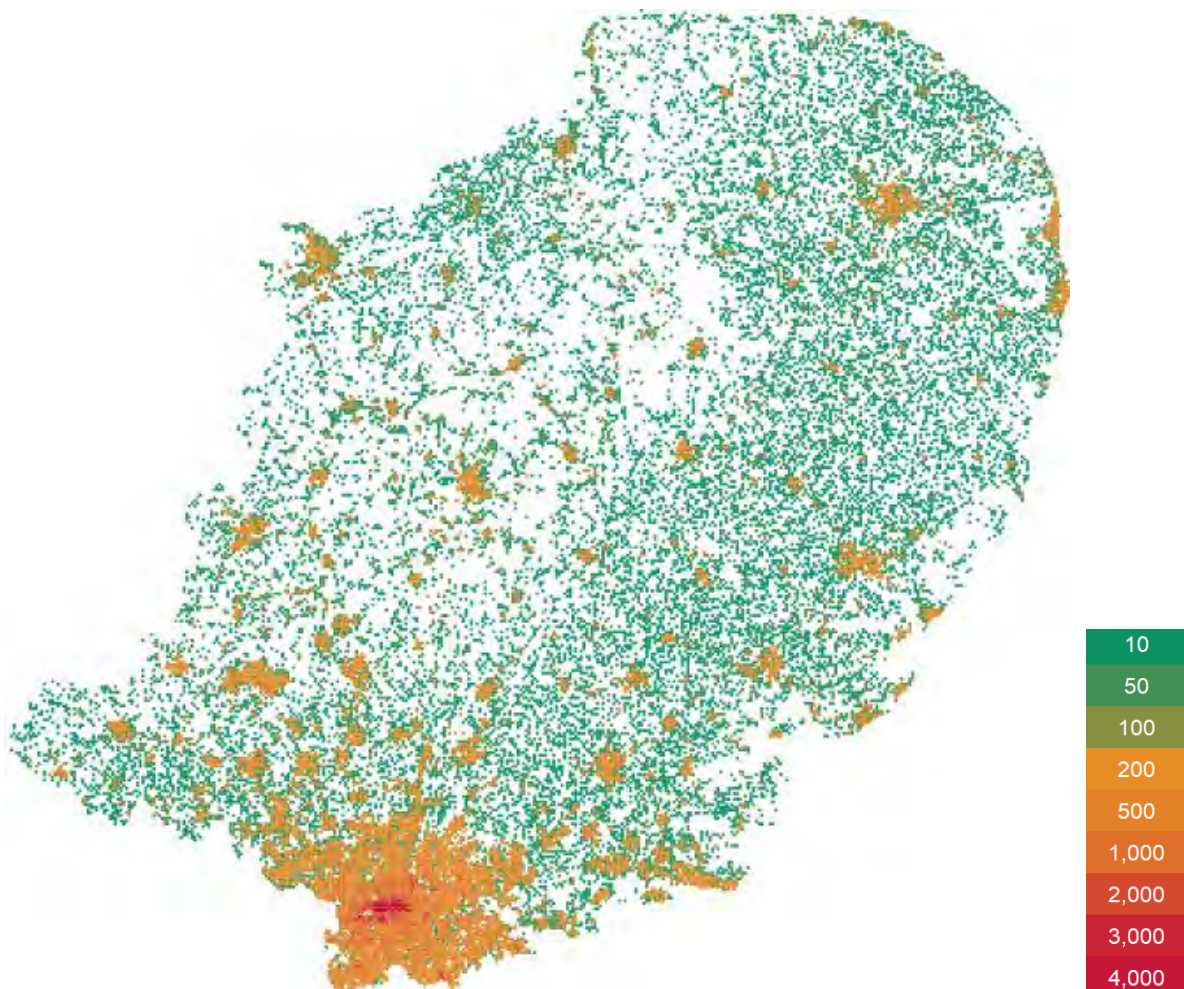
Figure 1.2: LPN and EPN service cables, low and high voltage networks and distribution transformer losses density in MWh/year.km 2
